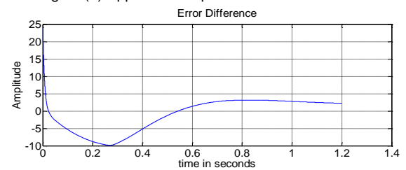
Fig. 18(c) Application of negative bias to the feedback
